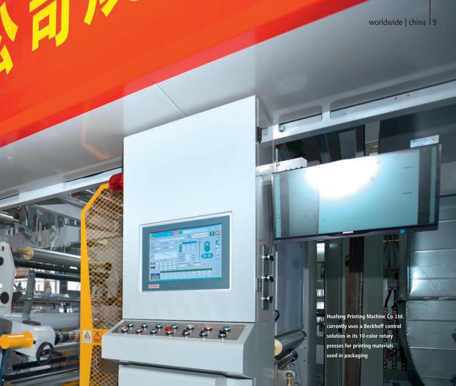
Huafeng Printing Machine Co. Ltd. currently uses a Beckhoff control solution in its 10-color rotary presses for printing materials used in packaging
