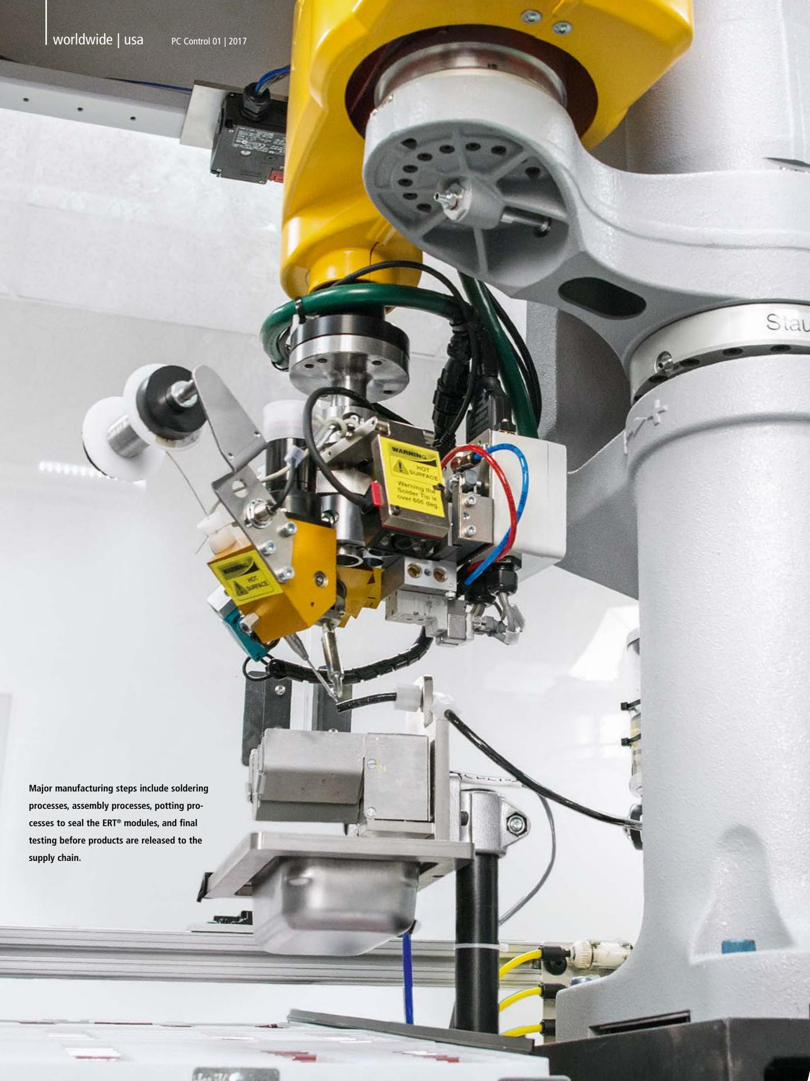
Major manufacturing steps include soldering processes, assembly processes, potting processes to seal the ERT® modules, and final testing before products are released to the supply chain.
