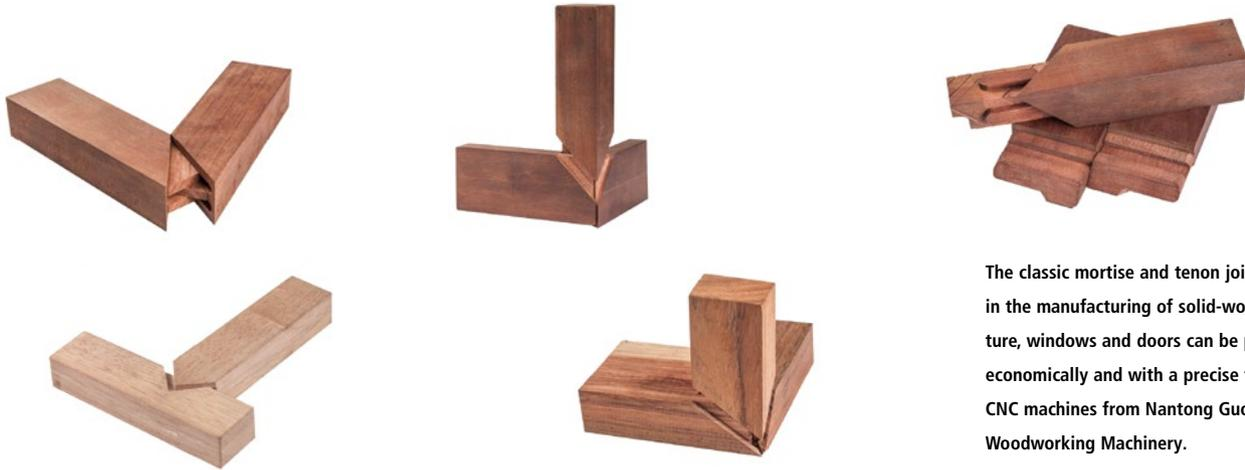
The classic mortise and tenon joints used in the manufacturing of solid-wood furniture, windows and doors can be produced economically and with a precise fit by the CNC machines from Nantong Guoquan Woodworking Machinery.
