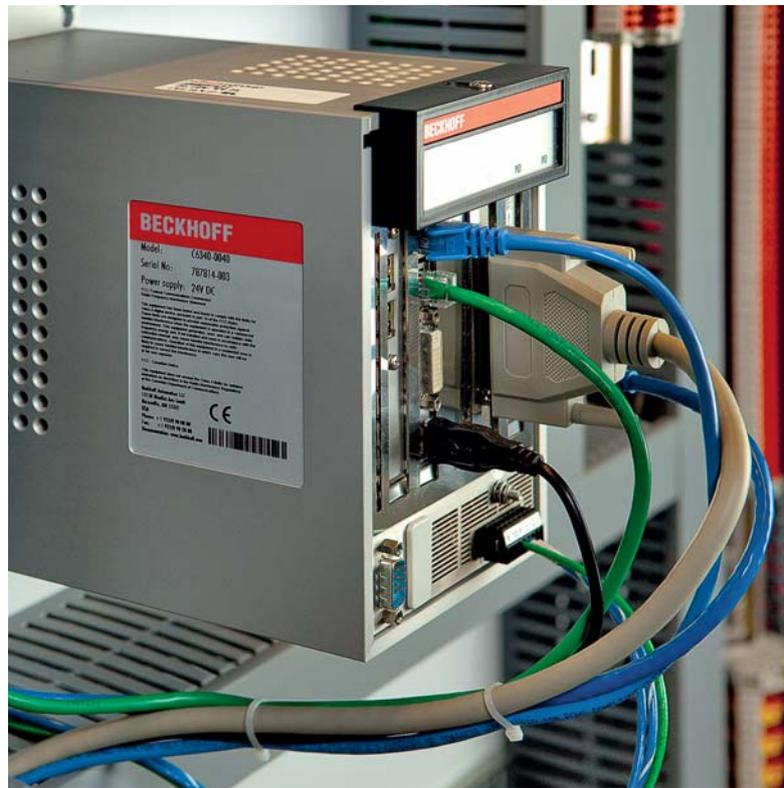
The backbone of the control system is a Beckhoff C6340 Industrial PC, equipped with an Intel® Pentium® M 1.8 GHz processor.
