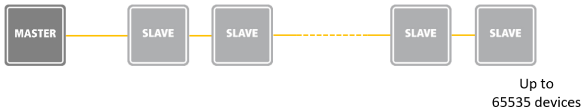
Figure 1: number of slaves on an EtherCAT network
