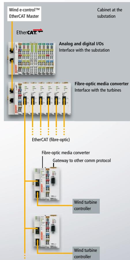
A general schematic diagram of the EtherCAT topology shows the functions handled by the individual modules in the wind farm.
