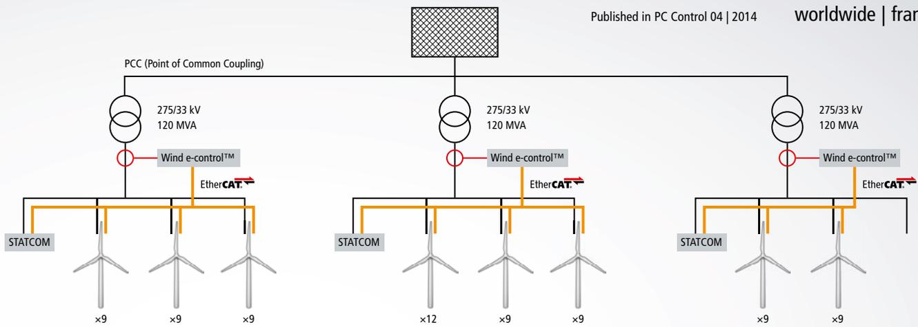
A Wind e-control™ system is provided for each transformer station, securing the EtherCAT data transmission between the individual wind turbines in the wind farm.
