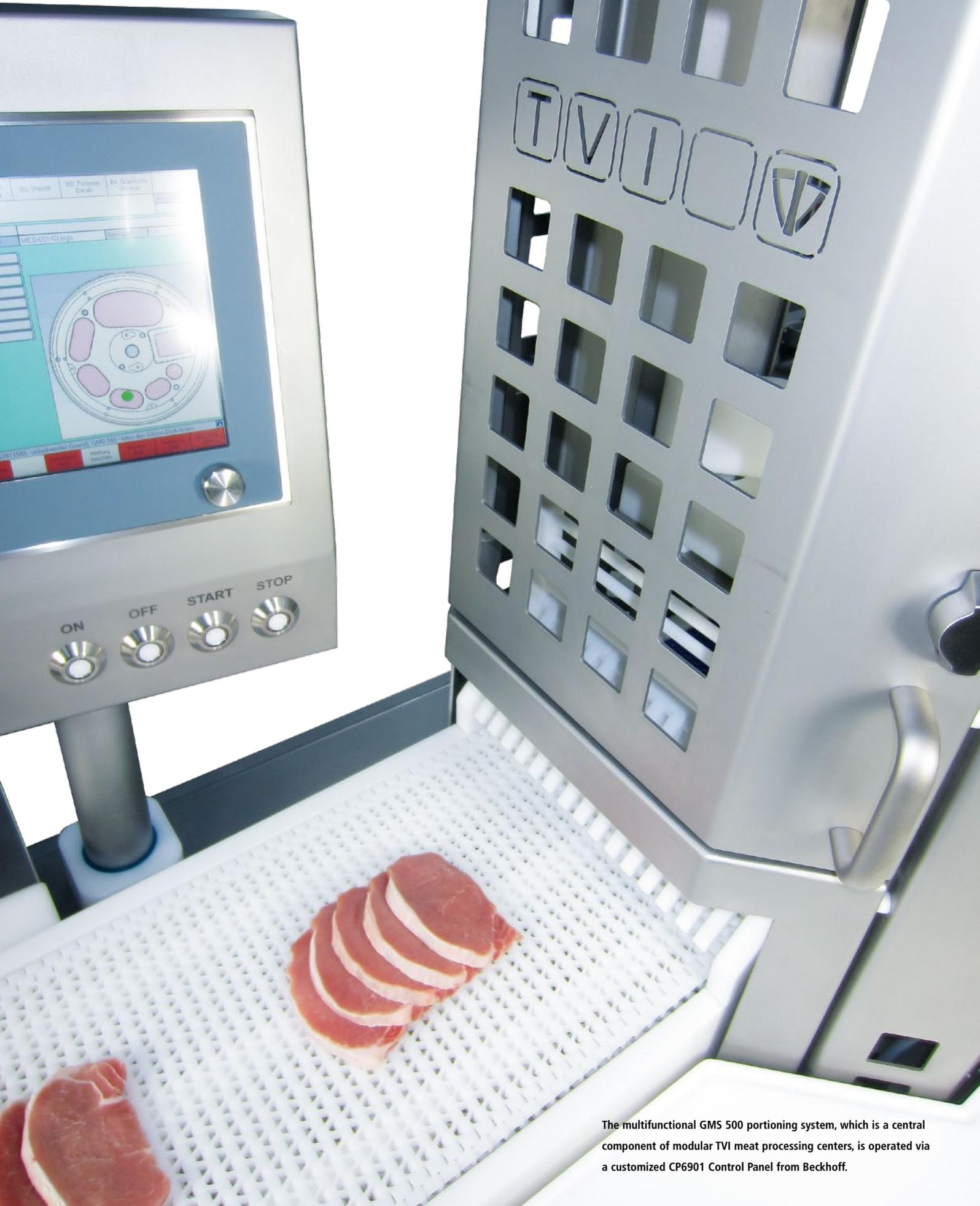
The multifunctional GMS 500 portioning system, which is a central component of modular TVI meat processing centers, is operated via a customized CP6901 Control Panel from Beckhoff.
