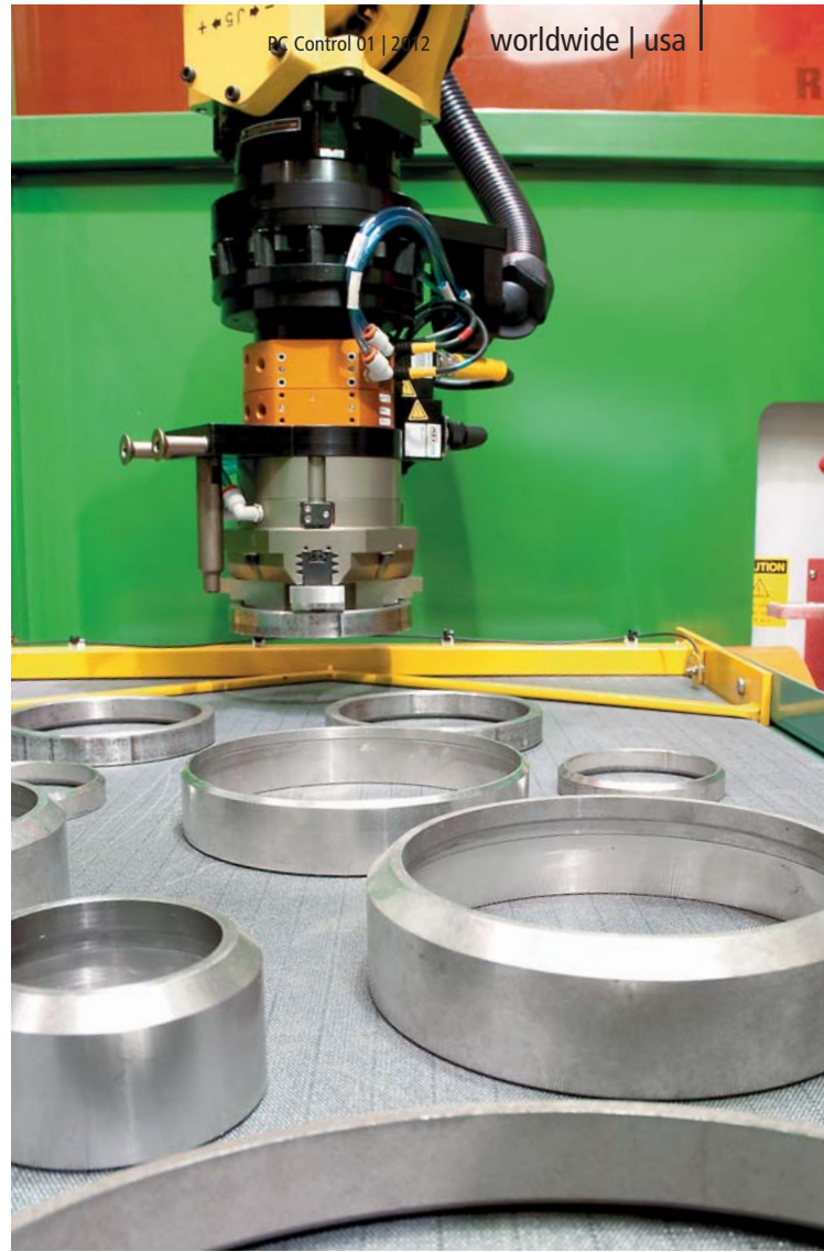
The robot picks up an end ring from an infeed conveyor.
