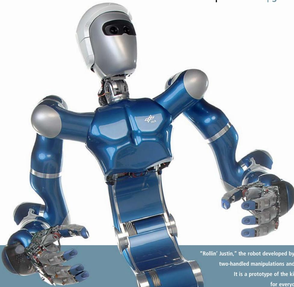
"Rollin' Justin," the robot developed by the German Aerospace Center (DLR), can perform complex, two-handed manipulations and can move freely about the room due to a mobile platform. It is a prototype of the kind of service robot that could be used in future households for everyday tasks or for fetching and bringing items in a warehouse.
