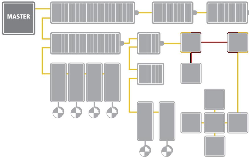
The topology flexibility of EtherCAT simplifies planning and installation.
