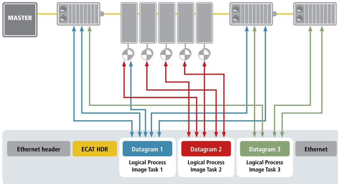
Process data is inserted and extracted on the fly: the unique functional principle of EtherCAT.
